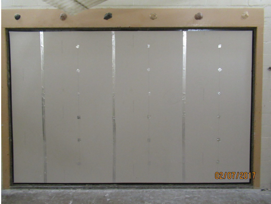
Figure 1 – Specimen mounted in the test opening.
