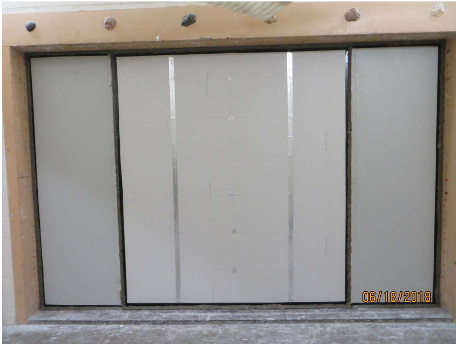
Figure 1 – Completed specimen mounted in test opening, as viewed from source room
