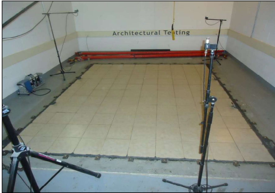
Source Room View of Test Specimen Installation
