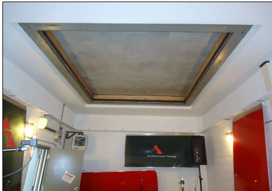
Receive Room View of Test Specimen Installation
