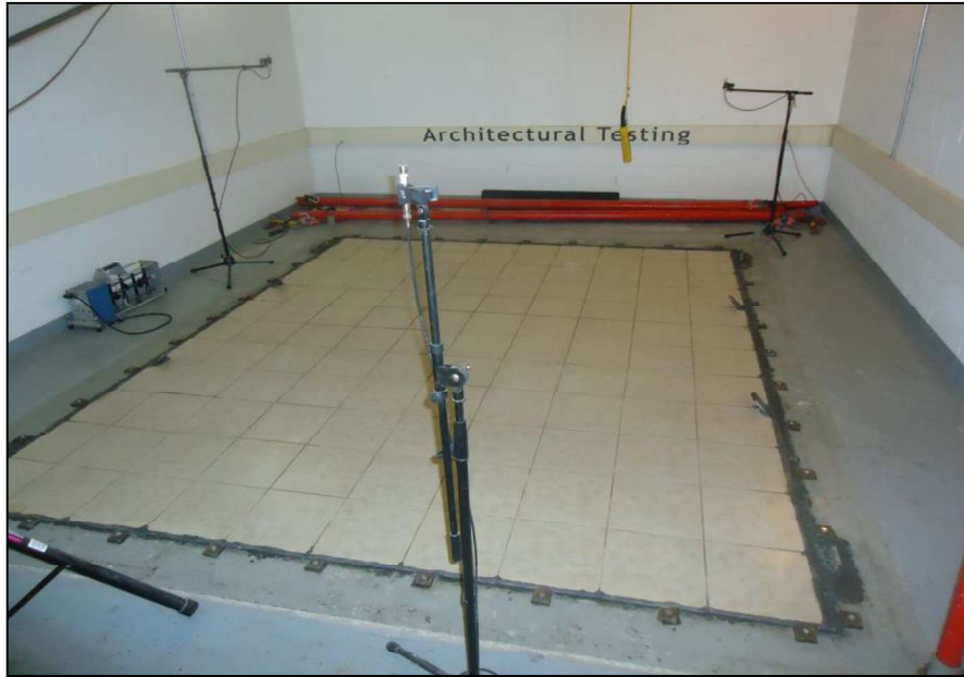
Source Room View of Test Specimen Installation
