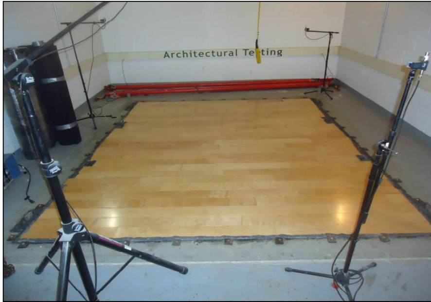
Source Room View of Test Specimen Installation
