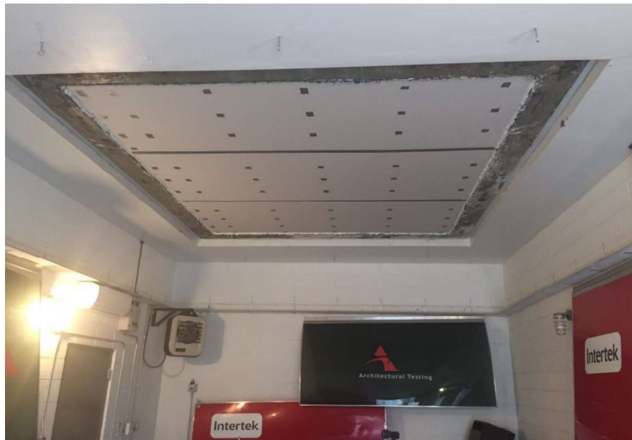
Receive Room View of Test Specimen Installation
