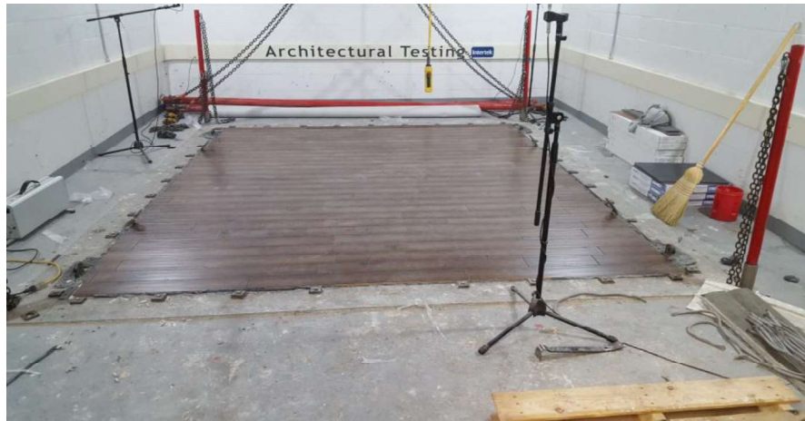
Source Room View of Test Specimen Installation
