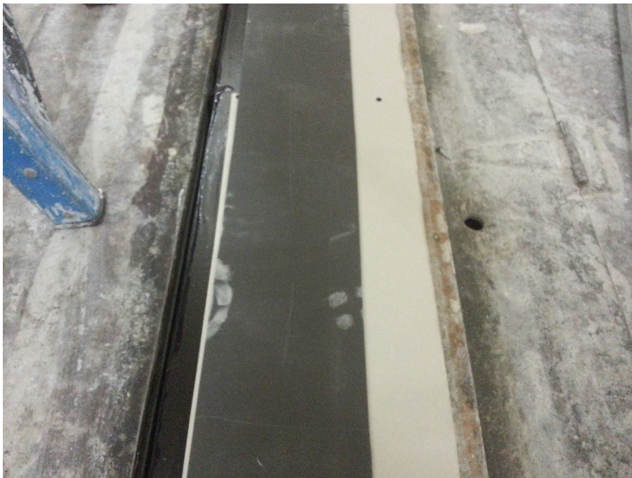
Figure 2 - Detail of Wall Blocker installed on test frame where the framing members will sit.
