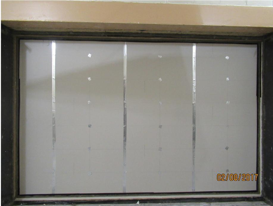
Figure 1 – Specimen mounted in the test opening.
