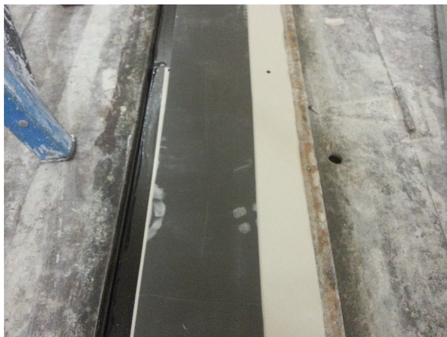
Figure 2 - Detail of Wall Blokker installed on test frame where the framing members will sit.
