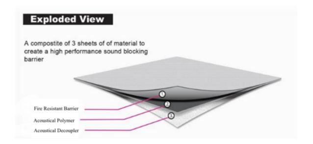
A Trio of layers combines a decoupling surface to the opposing face for improved sound reduction via transmission. Drop Ceiling Noise Blokker is an engineered ceiling tile accessory that installs on the plenum side directly on top of the tile. Acoustical Polymer & decoupler is manufactured from 100% post industrial and consumer materials. Laminated decoupling layer to eliminate sound transmission. Fire rated fiber scrim on exposed top.
