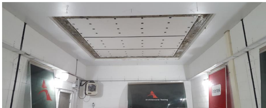
Receive Room View of Test Specimen Installation
