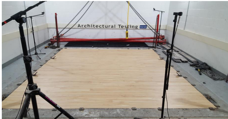
Source Room View of Test Specimen Installation
